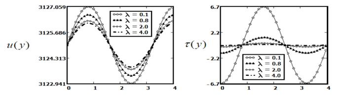
Figure 3. Profiles of the velocity field u(y,t) and the shear stress  $\tau(y,t)$  for Oldroyd-B fluid from equations (20) and (27), for  $\Omega_0 = 2$ ,  $\nu = 0.76$ ,  $\mu = 2.41$ ,  $\lambda_r = 3$ , t = 5 s,  $\alpha = 2$  and different values of  $\lambda$ .
