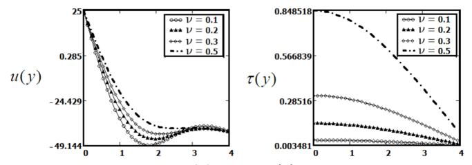
Figure 5. Profiles of the velocity field u(y,t) and the shear stress  $\tau(y,t)$  for Oldroyd-B fluid from equations (20) and (27), for  $\Omega_0 = 2$ ,  $\rho = 2.413$ , t = 5 s,  $\lambda = 2$ ,  $\lambda_r = 3$ , a = 2 and different values of  $v_{\perp}$ .
