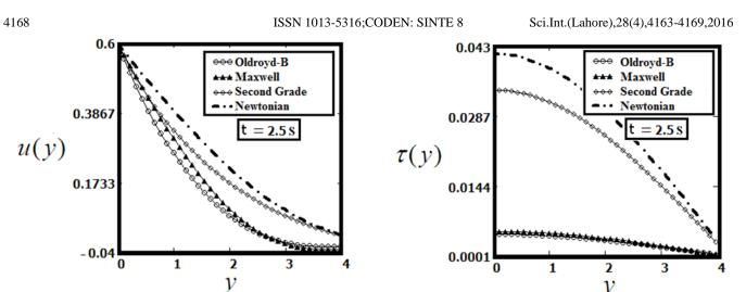
Figure 8. Profiles of the velocity fields u(y,t) and the shear stresses  $\tau(y,t)$  for Oldroyd-B, Maxwell, Second grade, Newtonian fluids from equations (20), (28), (30), (32), (27), (29), (31) and (33) for  $\Omega_0 = 2$ ,  $\nu = 0.76$ ,  $\mu = 2.41$ , t = 5 s,  $\lambda = 2$ ,  $\lambda_r = 3$ ,  $\alpha = 2$  and different values of t = 2.5 s.
