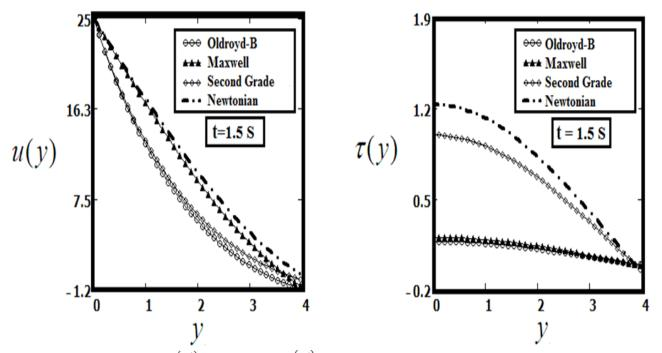
Figure 9. Profiles of the velocity fields u(y,t) and the shear stresses  $\tau(y,t)$  for Oldroyd-B, Maxwell, Second grade, Newtonian fluids from equations (20), (28), (30), (32), (27), (29), (31) and (33) for  $\Omega_0 = 2$ ,  $\nu = 0.76$ ,  $\mu = 2.41$ , t = 5 s,  $\lambda = 2$ ,  $\lambda_r = 3$ , a = 2 and different values of t = 2.5 s.
