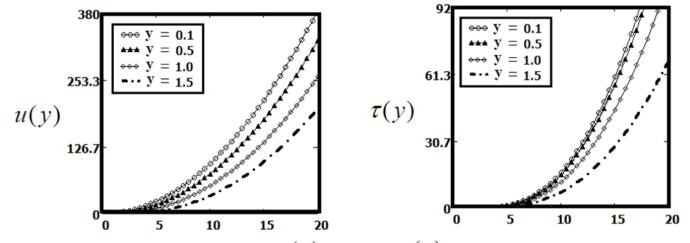
Figure 7. Profiles of the velocity field u(y,t) and the shear stress  $\tau(y,t)$  for Oldroyd-B fluid from equations (20) and (27) for  $\Omega_0 = 2$ ,  $\nu = 0.76$ ,  $\mu = 2.41$ ,  $\lambda = 2$ ,  $\lambda_r = 3$ ,  $\alpha = 2$  and different values of y.
