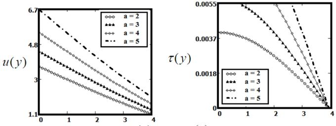
Figure 6. Profiles of the velocity field u(y,t) and the shear stress  $\tau(y,t)$  for Oldroyd-B fluid from equations (20) and (27), for  $\Omega_0 = 2, v = 0.76, \mu = 2.41, \lambda = 2, \lambda_r = 3, t = 2$  s and different values of a.
