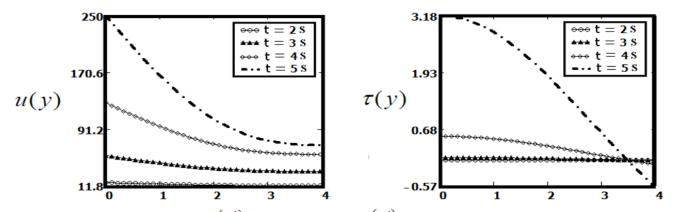
Figure 2: Profiles of the velocity field u(y,t) and the shear stress  $\tau(y,t)$  for Oldroyd-B fluid from equations (20) and (27) for  $\Omega_0 = 2, v = 0.76, \mu = 2.41, \lambda = 2, \lambda_r = 3$  a = 2 and different values of t.
